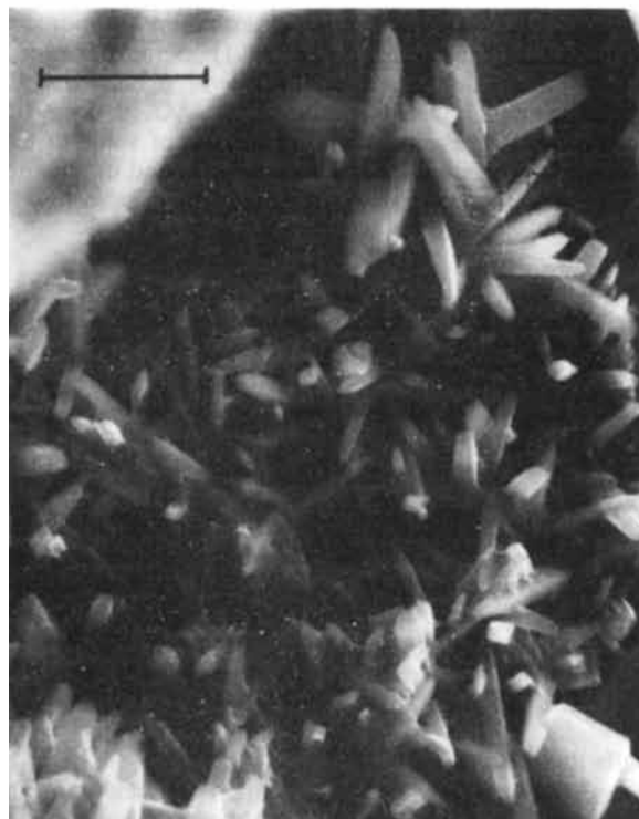
Figure 1. Hexagonal crystals of \beta - \text{Sb}_2\text{O}_4 containing ca. 5% vanadium formed from reaction of vanadium(v) oxide with antimony(III) oxide (scale bar = 10 \mu\text{m} )
